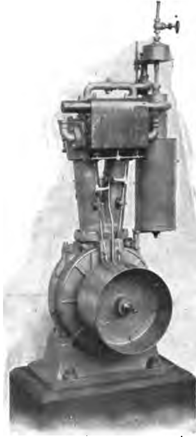
FIG. 304. —The Daimler V-shaped Gasoline Engine, with carburetter and parts attached. The object of constructing an engine with cylinders arranged as shown is to double the power capacity without correspondingly increasing the weight. This style of motor has been practically abandoned, and is no longer manufactured by the Daimler Companies.
